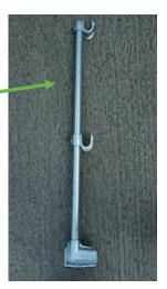
The locking collar goes into the first hole in the counterweight. The tube passes through the collar and is in position when the end of the tube is visible in the second hole. The setscrew on the locking collar is then tightened and the setscrews on the post base are tightened.
