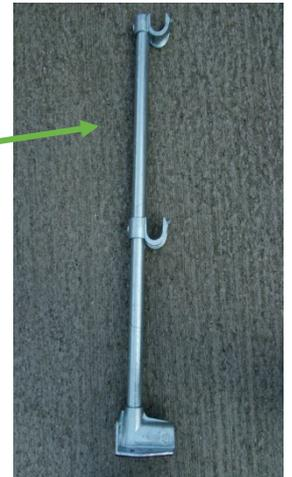
The locking collar goes into the first hole in the counterweight. The tube passes through the collar and is in position when the end of the tube is visible in the second hole. The setscrew on the locking collar is then tightened and the setscrews on the post base are tightened.
