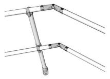
If you have a corner that is not quite 90°, you can use a D009 gradient change elbow as an obtuse or acute angle elbow as well. Ensure the tightening grubscrew is facing downwards to maintain a smooth rail. Unlike the 90° elbow, to use the D009 you will also need two of A09 internal joiners and four D797 sealing rings.
