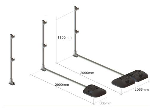
Lay out the equipment in approximately the positions shown below. Always ensure that you and the equipment are at a safe distance from the roof edge. It is recommended that this distance is no less than 2m.
